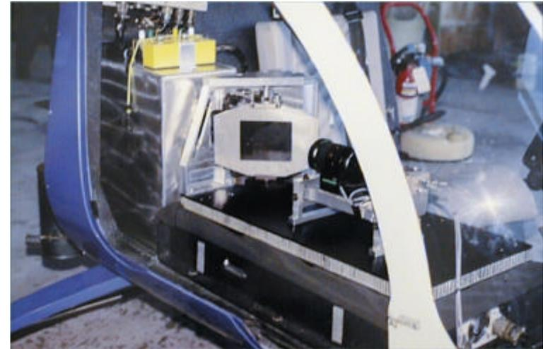
Camera System with Vibration Isolation
